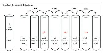
**Diagram 1:** Procedure of making dilutions.
