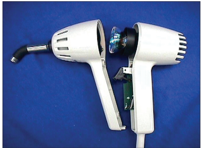
Figure 21: Maintenance by periodic visual inspection of unit such as filters and bulb
