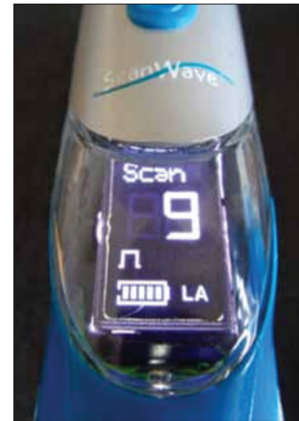
Figure 29: Display window showing operating mode (full scan), radiation time, battery status and Laser Target ring alignment aid activated for Scanwave by MiniLed
