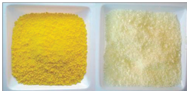
Figure 9: Camphorquinone (left) and Lucirin TPO (right)
