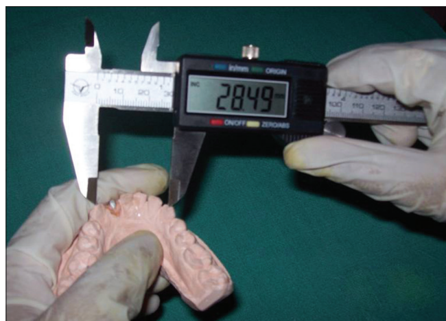
Figure 4: Measurement of intercanine width in mandibular cast
