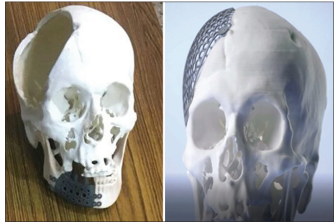
Figure 9: Cranioplasty and body of mandible implants in titanium fitted to a three-dimensional printed Selective Laser Sintering model
