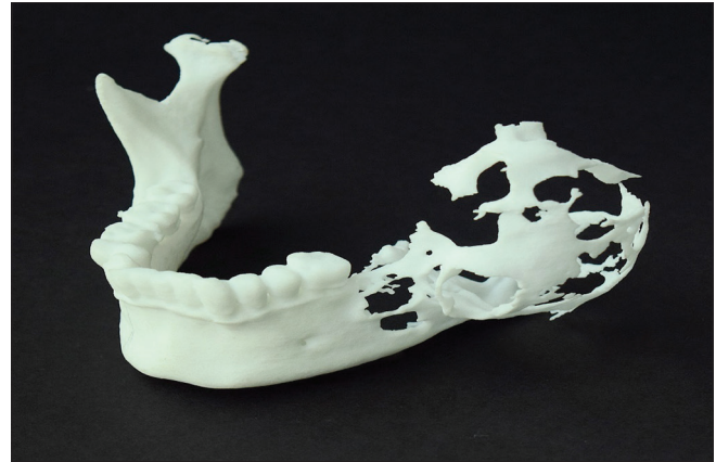
Figure 7: Three-dimensional-printed mandible model along with tumor made of Selective Laser Sintering on a Sinter Station HiQHS three-dimensional Systems machine. Material used is PA 12, biocompatible for in vivo applications
